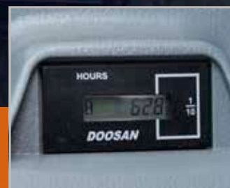
Hour meter (readable from ground level)
