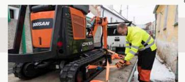
**Transportability:** The DX10Z fits easily on a conventional trailer. Easier transportability with new integrated upper structure tiedown points.
